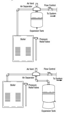
See next page for specifications and sizing information on Therm-O-Flex Space Heating Expansion Tanks.
