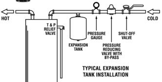
Expansion tanks are pre-charged with a 38 PSI air charge. If the inlet water pressure is higher than 38 PSI, the expansion tank's air pressure must be adjusted to match that pressure but must not be higher than 80 PSI.
